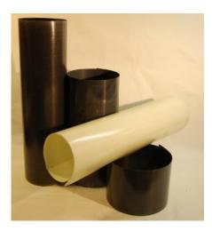
Figure 2. New laminates: carbon (black) and glass (white).
